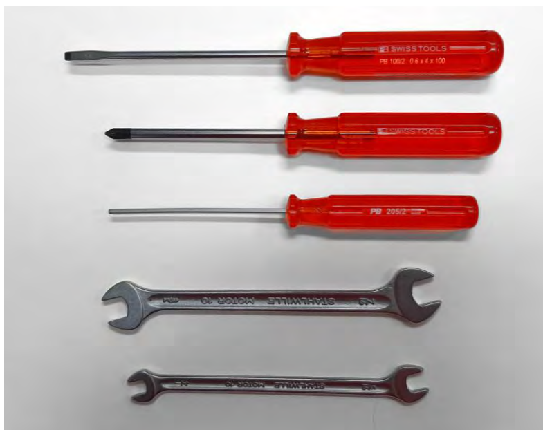
Figure 27 Minimum tools needed for standard maintenance and Synspec toolbox content list
