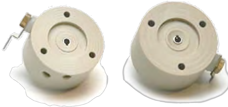
Figure 32 A good and eroded head
