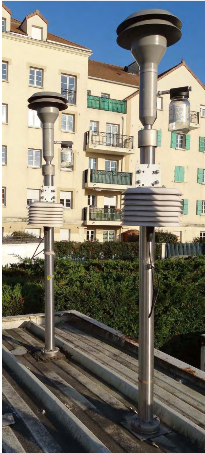
(1) PM10 sampling-dust head, (2) temperature and humidity sensor, (3) RST sampling line, (4) refer to Figure 1-10, (5) line part inside the room or the enclosure.
