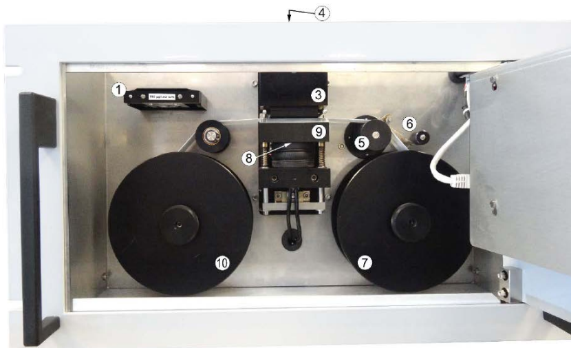
(1) reference gauge, (3) source holder, (4) retractable tip on sample inlet, (5) capstan, (6) pinch roller, (7) take-up reel, (8) Geiger-Müller detector tube, (9) plate assembly, (10) pay-out reel.
