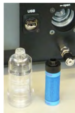
Figure 40: Filter and protective cover after removal
