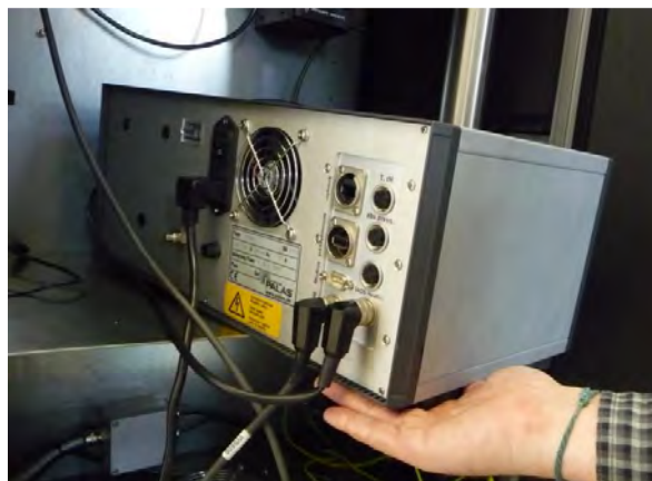
Figure 9: Connecting the weather station and IADS with the connections on the back
