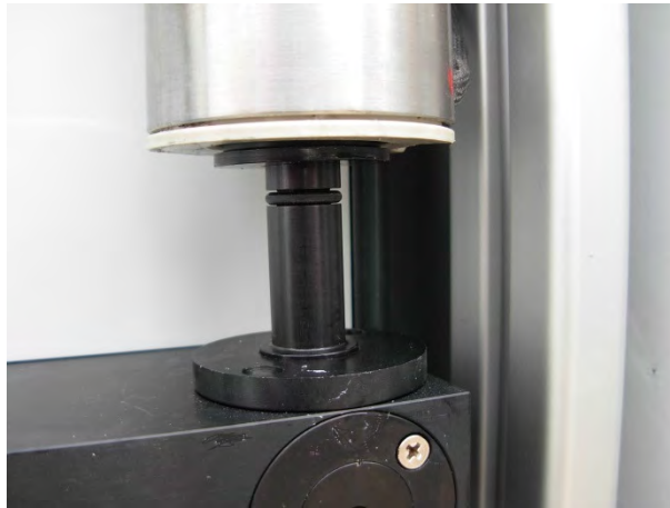
Figure 10: Connecting the sampling tube with the sampling inlet tube and the control unit
