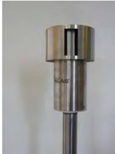
Figure 10: Sigma-2-sampling head for the Fidas ® 200 S / Fidas ® 200
