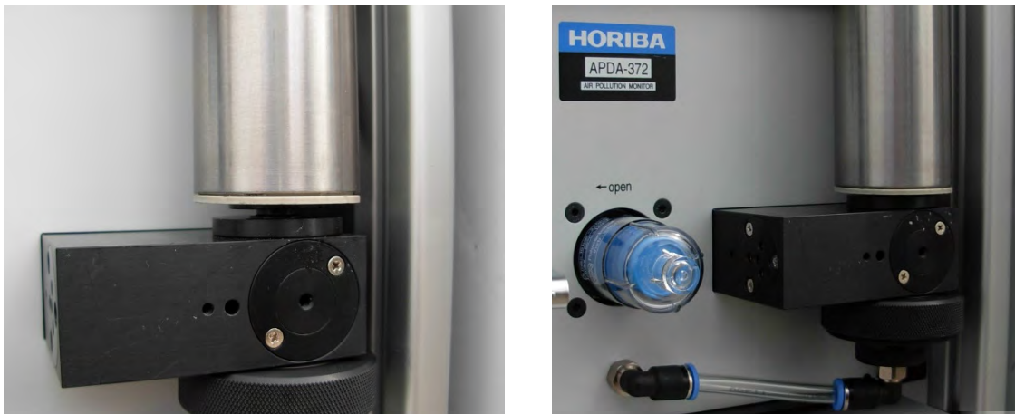
Figure 11: Incorrect position of sampling tube shown on left, correct position on right
