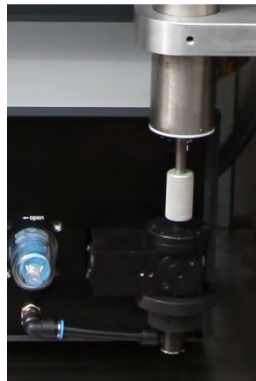
Figure 31: Connection of the sensor inlet with IADS humidity compensation module
