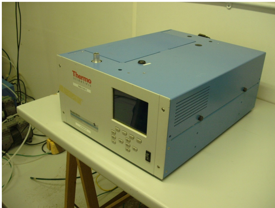
Figure 6: Model 5014i Beta measuring system – here as Model 5030i SHARP after disassembly of the nephelometer module
