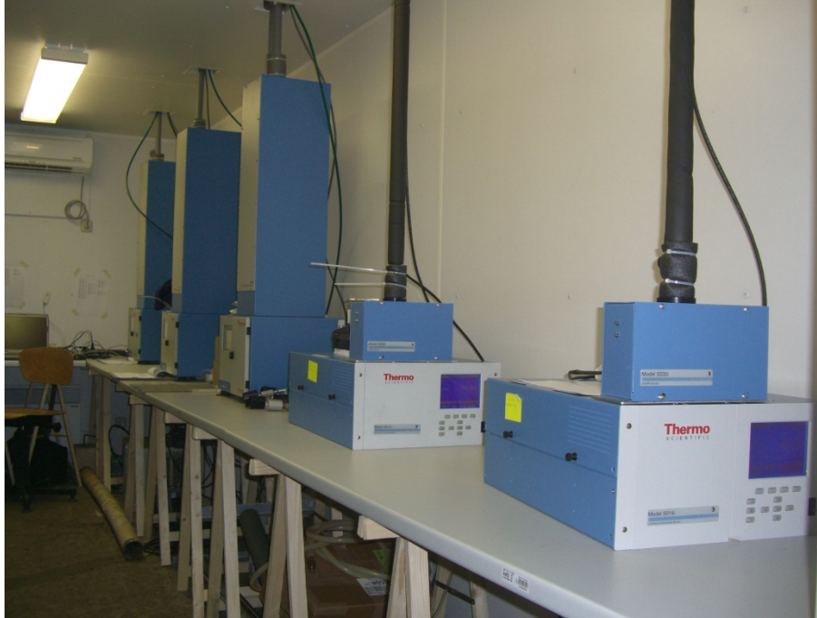
Figure 7: Model 5014i Beta measuring system (Systems 1 and 2 from right) at measuring station – here as Model 5030i SHARP with nephelometer module
