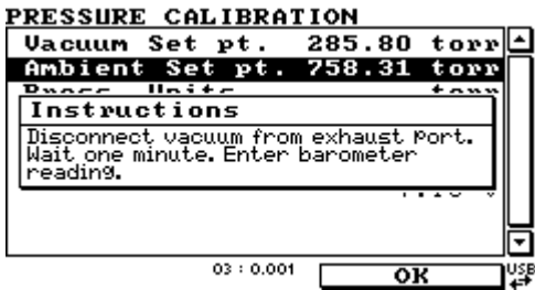
Figure 32 – Ambient set point calibration screen
