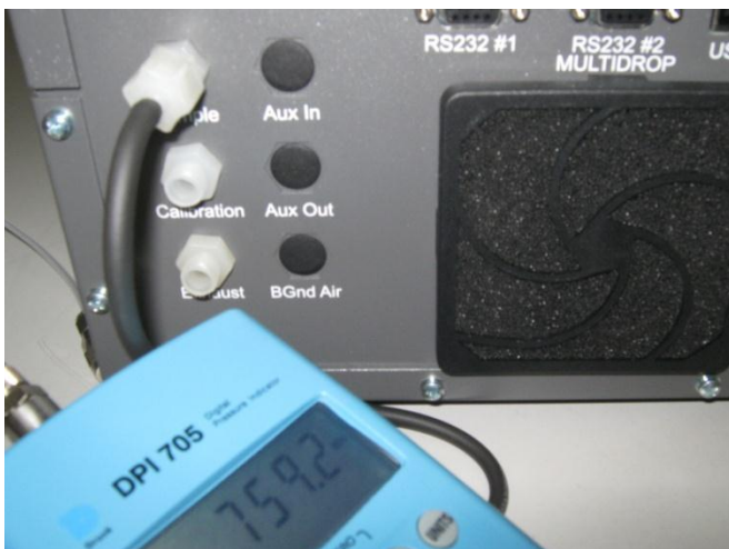
Figure 29 - Pressure calibration; external pressure meter
