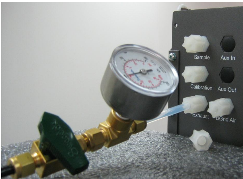
Figure 38 – Pressure gauge on exhaust
