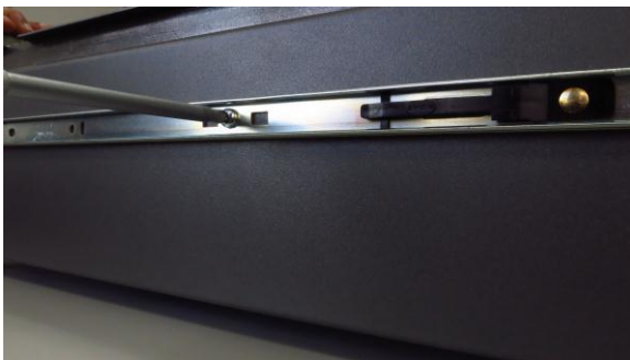
Figure 48 - Assemble inner slide on chassis
