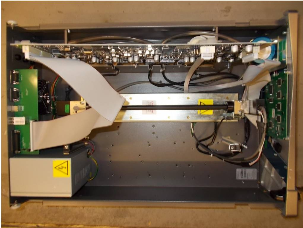
Figure 4: Internal view of the Serinus 10 measuring system
