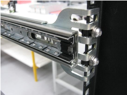
Figure 50 - Assemble inner slide on chassis
