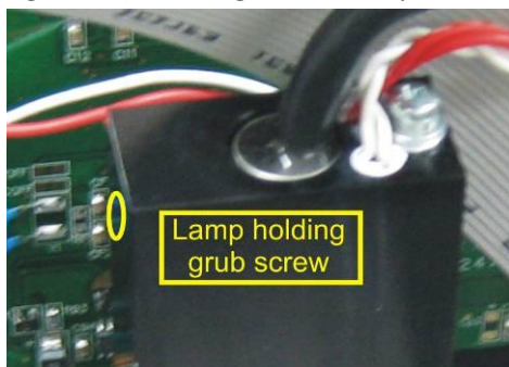
Figure 39 - Location of UV lamp fastening grub screw
