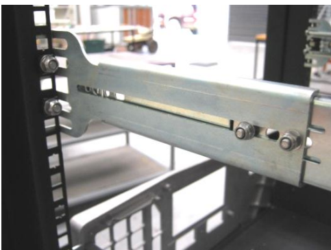
Figure 51 - Attach rack mount adaptors to outer slides
