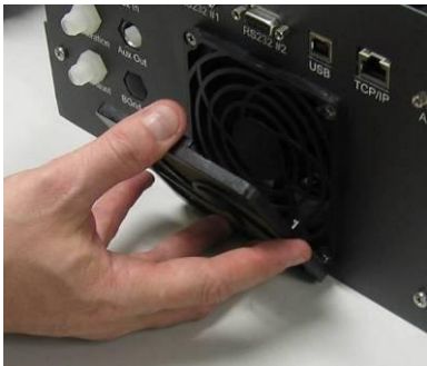
Figure 37 - Removing fan filter
