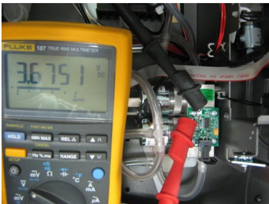
Figure 42 – Typical test point reading of cell pressure sensor.
