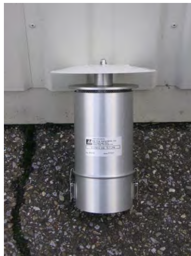
Figure 4: European PM10-sampling inlet BX-809 for BAM-1020
