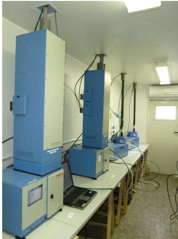
Figure 7: Measuring device TEOM 1405-F Ambient Particulate Monitor (1 st system from left) in measuring station
