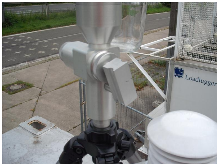
Figure 4: PM 2.5 Sharp Cut Cyclone for TEOM 1405-F Ambient Particulate Monitor
