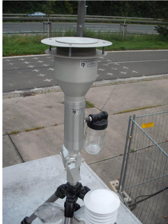
Figure 3: American PM 10 -sampling inlet (Original style, p/n 57-000596-0001) for TEOM 1405-F Ambient Particulate Monitor
