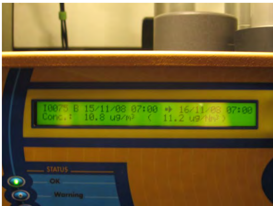
Figure 36: Display for measured values, Line B (PM 2.5 ), data recall from buffer to display
