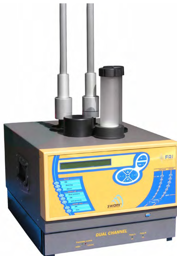
Figure 4: SWAM 5a Dual Channel Monitor measuring system
