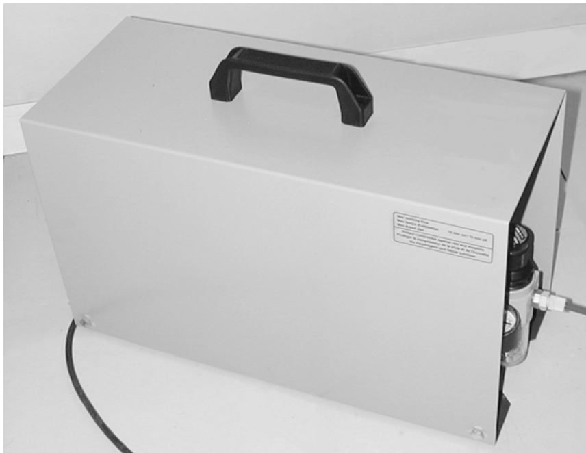
Figure 6: Service air compressor unit
