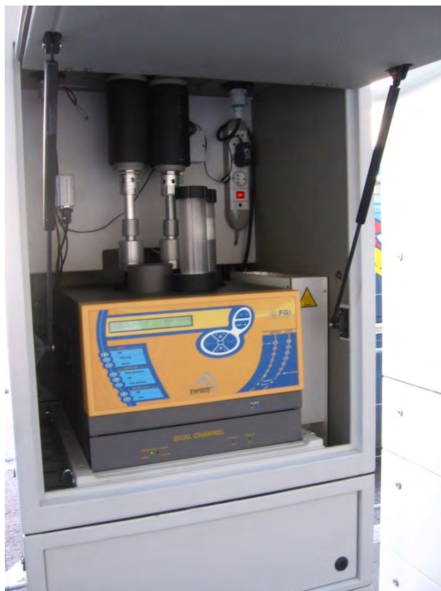
Figure 12: SWAM 5a Dual Channel Monitor inside the outdoor measurement rack
