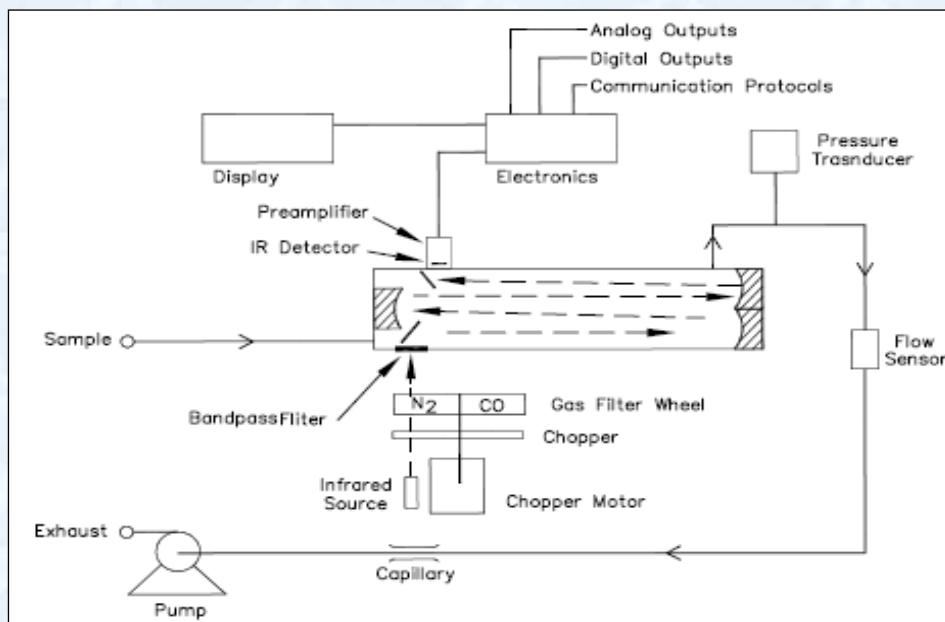
The measuring principle complies with the standard reference method as stipulated in EN 14626.
